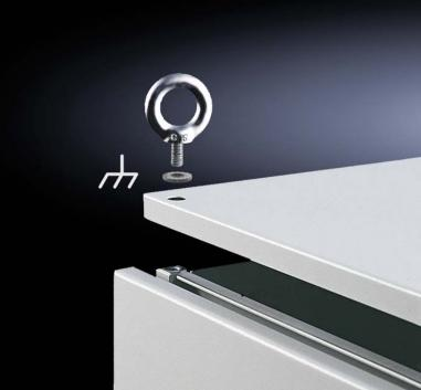
Potential equalisation for the gland plates, side panels, rear panel and roof is achieved automatically when the enclosure is assembled. That guarantees a conductive contact between the frame and all panel parts. Where there are no electrical devices mounted on the panel parts, it is possible to forego earth straps.
